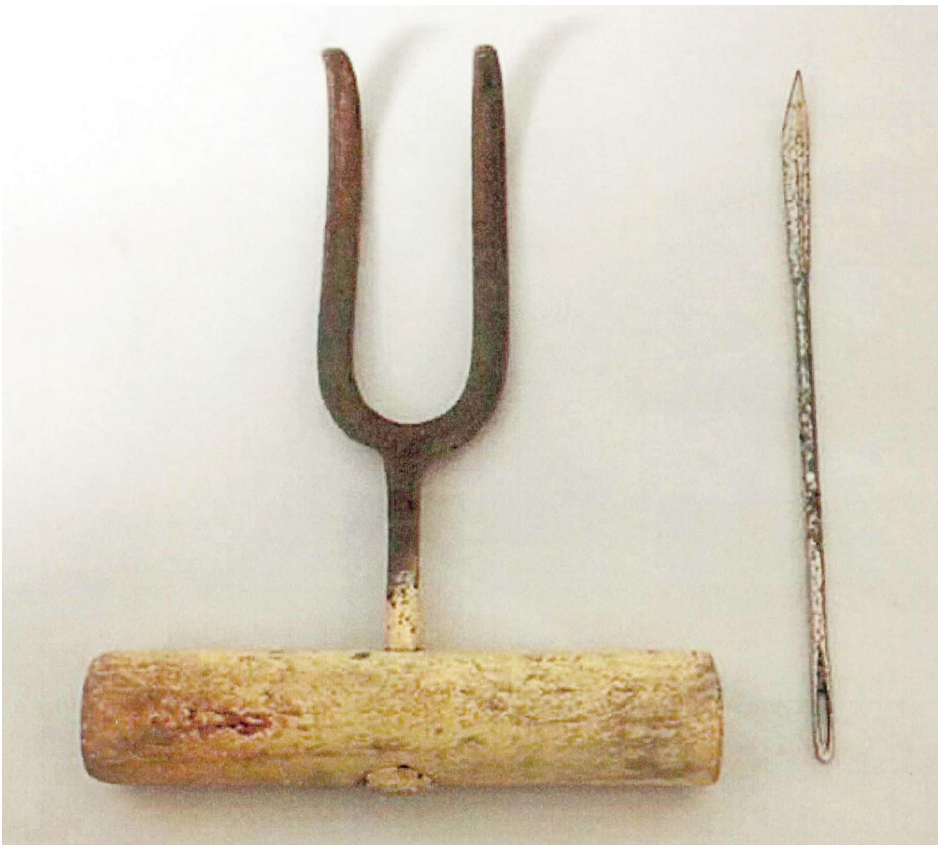
Figure 3: Clem O'Loughlin's hook and his brother's (Michael O'Loughlin) needle for bag sewing.
